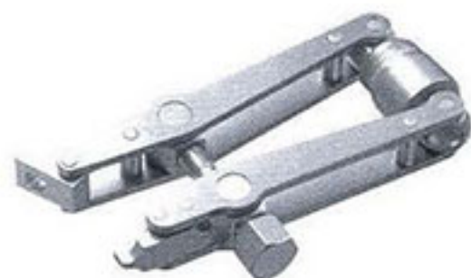
321.120 Tension Device, articulated span 20mm, can also be used as a distractor. Colour scale: yellow up to 500N, green up to 1000N, red above 1000N
