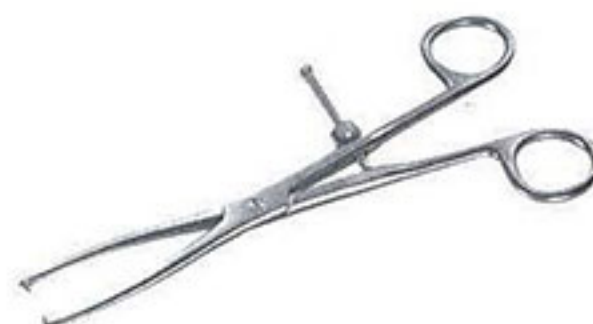
399.170 Malleolar Forceps length 210mm, with 2 points meeting at a 15° angle, speed lock
