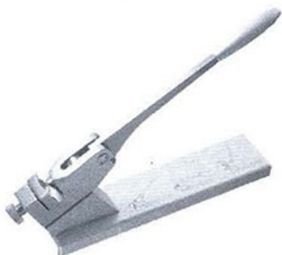
329.300 Bending Press length 400mm
