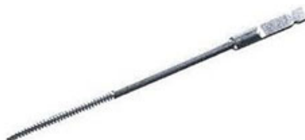
311.260 1 Tap for 2.7mm Cortex Screws total length 100mm, thread length 33mm predrilling: 2.0mm dia.
