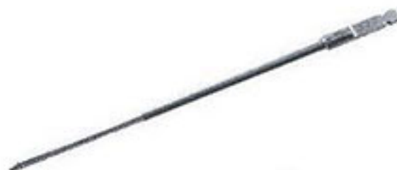
311.280 1 Tap for 2.7mm Cortex Screws total length 125mm, thread length 40mm predrilling: 2.0mm dia.
