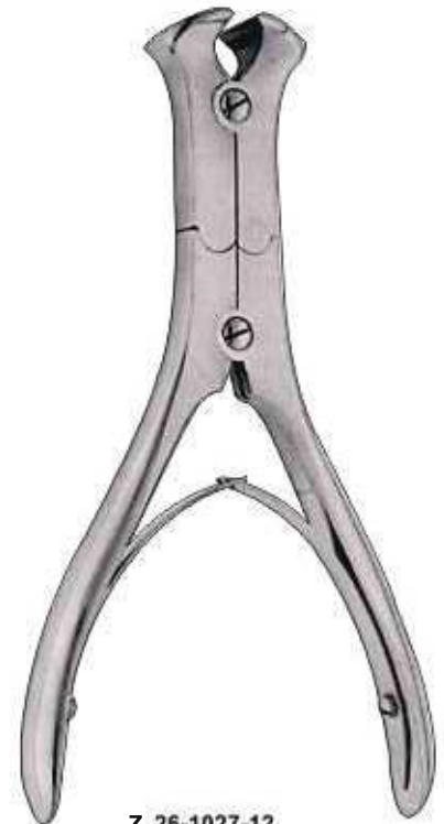
Z-26-1027-12 Wire Cutter soft wire 2.0 mm hard wire 1.2 mm
